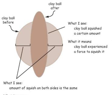
**Caption:** This sketch shows how a clay ball behaves when it is "squeezed" in a collision. The ball shows the same amount of squish on both sides, so the amount of force is equal. The difference is the forces are in opposite directions.
